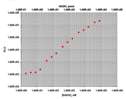
Fig. 1. Calibration curves (log-log plot) for NADH obtained using Highly Pure Bacterial Luciferase (50µg/ml, NovoCIB, E-Nov 10).
